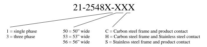
The machine is completed with choice of electrical package. See Section 8
